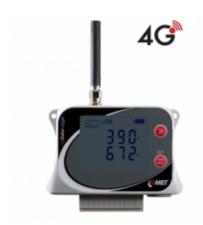
Datalogger is designed to record temperature from three thermocouples, one Pt1000 probe and one internal temperature sensor. In case of exceeded set limits, SMS and JSON messages can be sent via 4G data connection. Measured values can be sent to the internet storage <a href="COMETCloud">COMETCLOUD</a>, which is a complete monitoring, alarm and analysis system.
