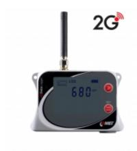
GSM datalogger is designed to record CO2 from built-in sensor. In case of exceeded set limits, SMS and JSON messages can be sent via GPRS data connection. Measured values can be sent to the internet storage <a href="COMETCloud">COMETCLOUD</a>, which is a complete monitoring, alarm and analysis system.
