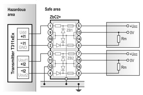
**Warning:** the value of the supply voltage +Ucc must not exceed the value of the maximum allowed working voltage of the Zener barrier (Uwmax = 26 V)
