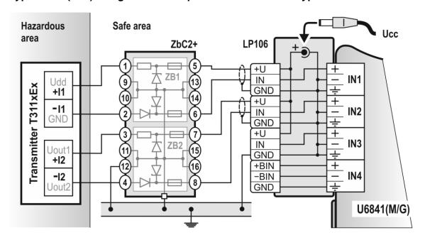
**Warning:** the value of the supply voltage Ucc must not exceed the value of the maximum allowed working voltage of the Zener barrier (Uwmax = 26 V). Use a stabilized ac/dc adapter A1941 (24Vdc).
