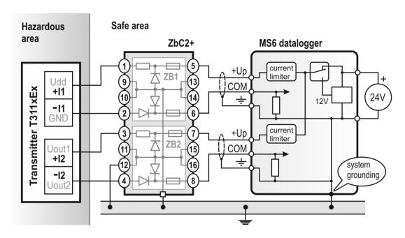
**Warning:** the supply voltage of the datalogger MS6 must not exceed the value of the maximum allowed working voltage of the Zener barrier (Uwmax = 26 V). Use a stabilized 24 Vdc power supply from the recommended accessory (unstabilized ac/dc adapter A1759 is not suitable for power supply).
