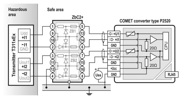
**Warning:** the value of the supply voltage +Uss must not exceed the value of the maximum allowed working voltage of the Zener barrier (Uwmax = 26 V). Use a stabilized 24 Vdc power supply from the recommended accessory.
