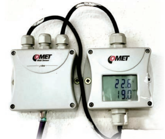
P2520 - current loop output and conversion to IT protocols
